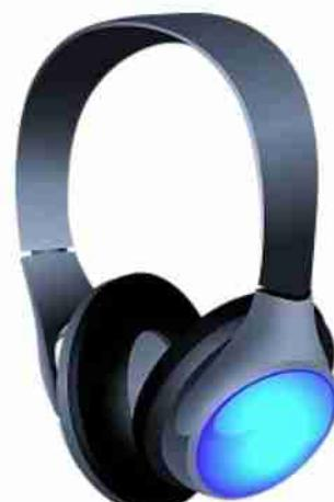
➤ The headphone is a type of output device with small speakers on the left and right. When we connect it to our CPU, the output sound of the computer starts coming from this headphones, so that we can hear it easily by plugging it into the ears.
