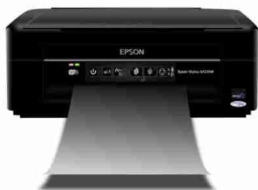
❖ In such printers, ink is used to print any letter or picture that is filled into the cartridge. When that ink is on the paper as a spray, it is printed. Its speed is not very high; it is copied in about 15-20 seconds.
